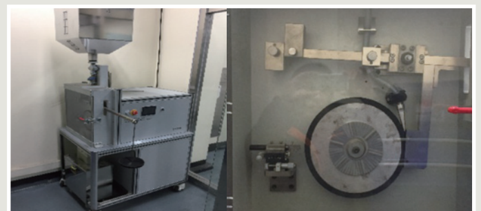
▲ ASTM G65 Sand Abrasion Test
